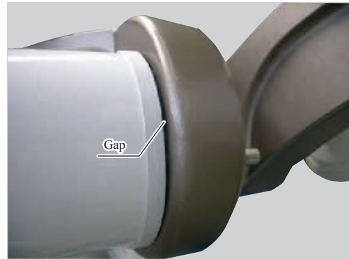
Gap at top of cover
