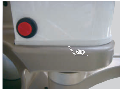
Gap at bottom of cover
